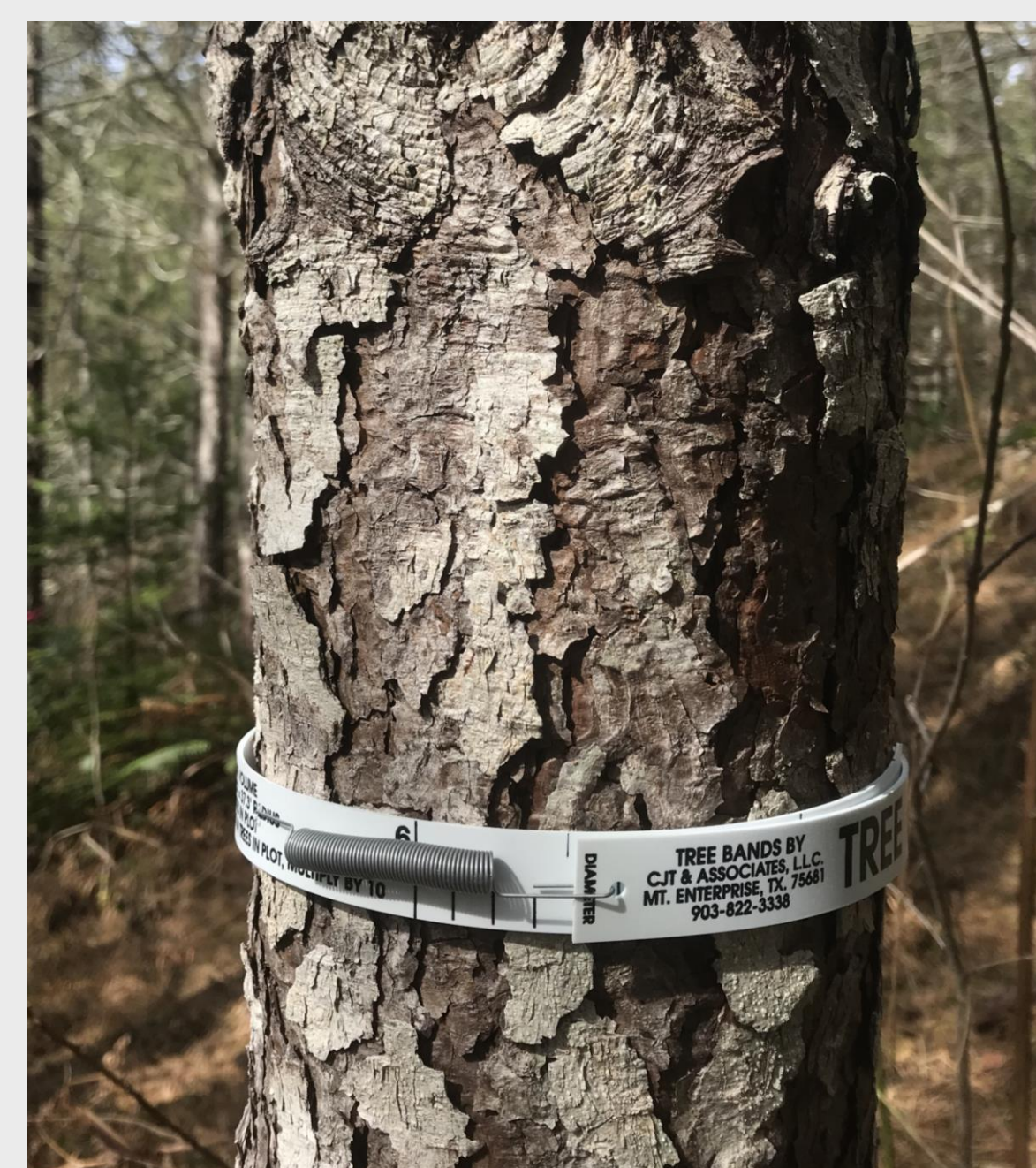
Figure 3. Dendrometer band on a Willamette Valley ponderosa pine.
